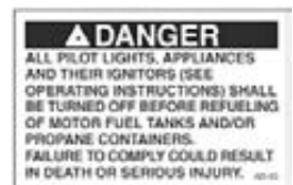
“Shut off for re-fueling” Label
