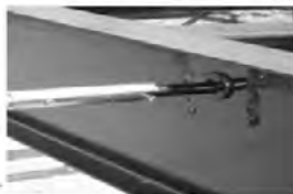
Fig. 2-Through Frame Crank Extension w/Pin
