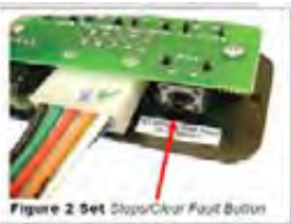
Figure 2 Set Stops/Clear Fault Button
