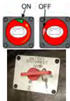
Battery Disconnect Switches
